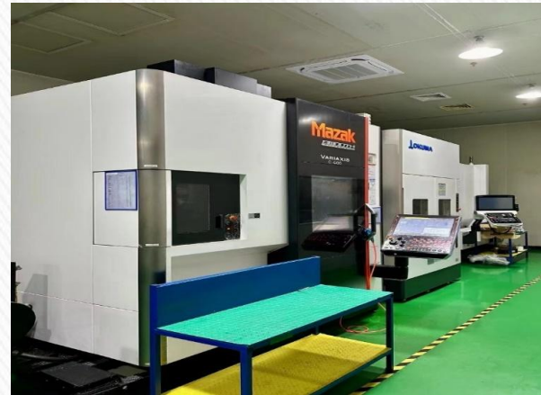
Mazak 5 Axis CNC Accuracy +/- 0.002 mm
